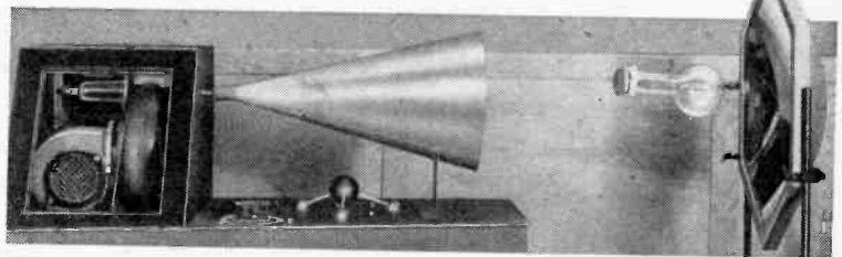
G.E.C. set-up for detecting mm waves using an ammonia filled flask.
